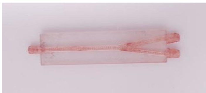
Fig. 1: 3D-printed microfluidic channel incorporating sol-gel pH sensing film.
